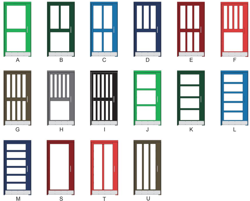
Please note, the configurations are shown with glazing panels, but any of these may be replaced with solid infill. 6mm or 10mm laminate, polycarbonate or double glazing is available in our Classic<sup>AL</sup> design. Alternative designs are available with the Classic2 steel communal doors and Classic2<sup>S</sup> stainless steel doors.
